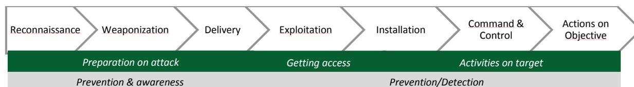
Figure 2 Seven stages of a cyber-attack, with the red team and blue teams main tasks
